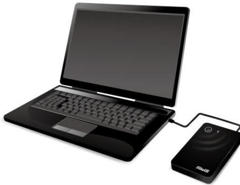
**Fig. 1** Connect H10 to your computer by USB 3.0 cable
